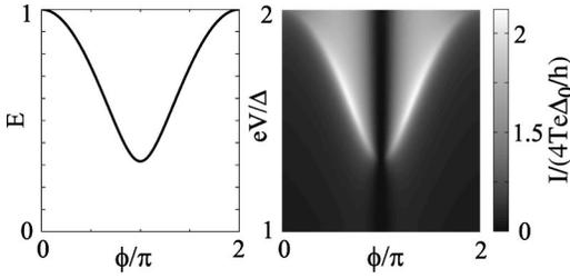
FIG. 6. Left: the energy of the (positive) Andreev level for  $D = 0.9$ , as a function of the phase difference. Right: the current peak (light region) at  $eV \approx \Delta + E_a(\phi)$  follows the position of the Andreev level.
