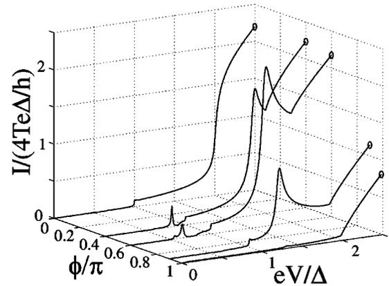
FIG. 5. The current-voltage characteristics at zero temperature of an interferometer with  $2T = 0.08$ ,  $R = 0.1$ , and  $\phi = 0, \phi = 2\pi/5, \phi = 3\pi/5, \phi = 0.9\pi$ , and  $\phi = 0.99\pi$ .
