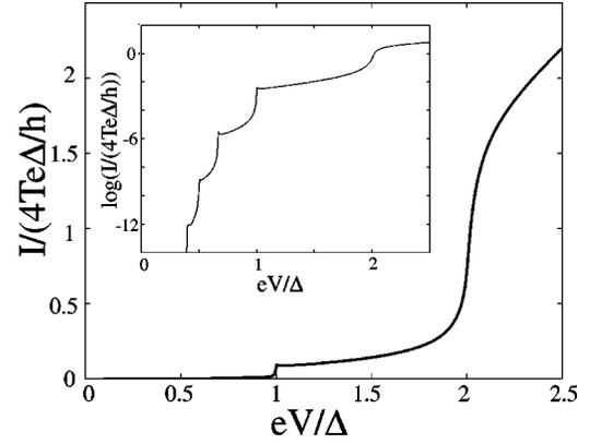
FIG. 4. The subharmonic gap structure of a superconducting point contact with current steps  $eV = 2\Delta/n$ ,  $n = 1, 2, 3, \dots$  (most visible on the logarithmic diagram). The transmission probability of the point contact is  $T_{PC} = 0.08$ , which corresponds to an SNS interferometer with  $\phi = 0$  and  $2T = 0.08$ .
