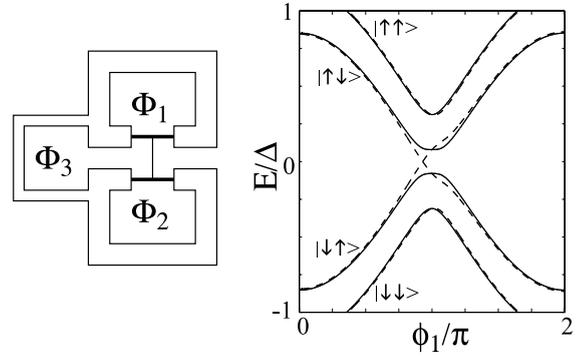
Fig. 3. Left: Coupling of ALQs by means of a four terminal quantum contact. The flux  $\Phi_3$  through the third superconducting loop can be used to control the coupling. Right: The two particle spectrum of two interacting ALQs,  $D_1 = D_2 = 0.97$ ,  $T = 0.01$  and  $\phi_2 = 0.93\pi$ . The solid line corresponds to coupled qubits ( $\phi_3 = \pi/2$ ) and the dashed line corresponds to uncoupled qubits ( $\phi_3 = 0$ ).
