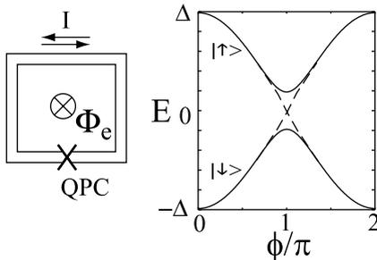
Fig. 1. Left: Sketch of the ALQ—a non-hysteretic rf SQUID with a QPC. Right: The energy spectrum of the QPC with finite reflectivity ( $R = 0.04$ ) (—), appears as a hybridization of the current states  $|\uparrow\rangle$  and  $|\downarrow\rangle$  ( $R = 0$ ) (---).
